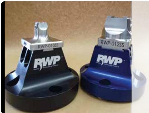
Clamping fixtures mounted to clamping fixtures extend the modularity of the Raptor system.
