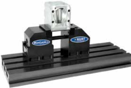
High-profile vises such as Kurt's Maxlock 350 are designed so that clamping forces are applied near the workpiece surface. It is shown here mounted on a T-slot table with optional risers.
