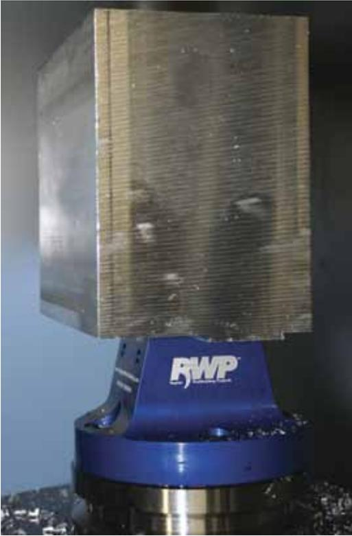
A “dovetail strip” on the underside of the blank workpiece interfaces with the dovetail features on the fixture. The Raptor RWP-001 pedestal fixture has a dovetail slot 1.5 inches wide. The blank measures about 4 inches wide, 6 inches long and 7 inches high and produced the part shown on page 82.
