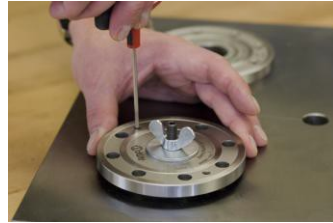
Uniform insertion of 4 opposing cylinder screws (2), up to flat contact.
