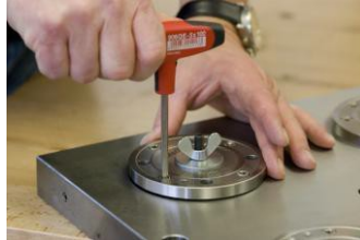
Insert assembly tool (5), loosen cylinder screws (2) evenly
