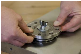
Uniform and tilt-free extraction of the clamping system
