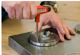
Uniformly loosen cylinder screws
