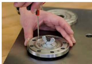
Screw in threaded stud in order to be able to press the clamping system down
