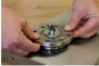
Uniform and tilt-free removal of the clamping system
