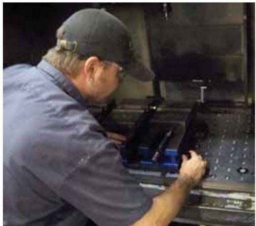
CNC machinist Ricky Goble secures a fixture using the Ball Lock system. Tightening shanks by hand saves time, locking and locating the fixture in one motion.
