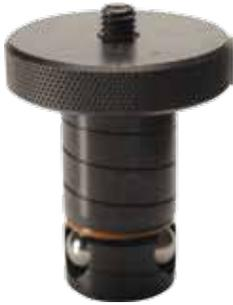
The Ball Lock system operates with three primary components: shanks, liner bushings and receiver bushings. The shank extends through the liner bushing in a fixture plate and into the receiver bushing to locate and secure the fixture.
