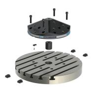
Mount direct to t-slotted machine table. Locate with center pin and timing key. Secure to table with t-nuts & SHCS
