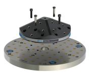
Mount to Fixture-Pro® base elements such as subplates via Jergens QLS Mounting System. A combination of (2) 12mm QLS shoulder screws and (2) M12 SHCS will accurately locate and securely clamp the pyramid to a base element.
